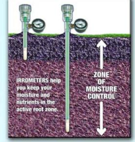
This two IRROMETER sensing station shows a wet reading (30 cb) at the lower depth and a dry reading (60 cb) at the shallower depth. Therefore, a short irrigation is needed.
